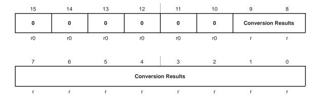
**Conversion** Bits The 10-bit conversion results are right justified, straight-binary format. Bit 9 is the MSB. Bits 15-10 are always 0.
